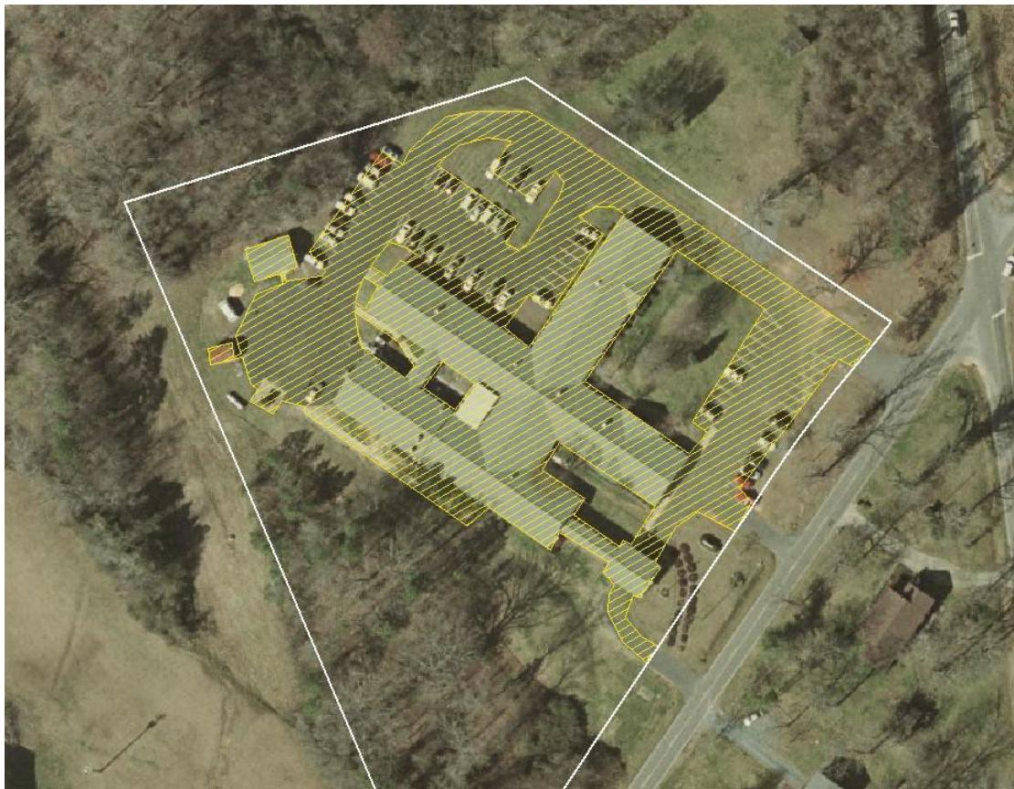
82,550 square feet of impervious surface area (impervious area shaded)
