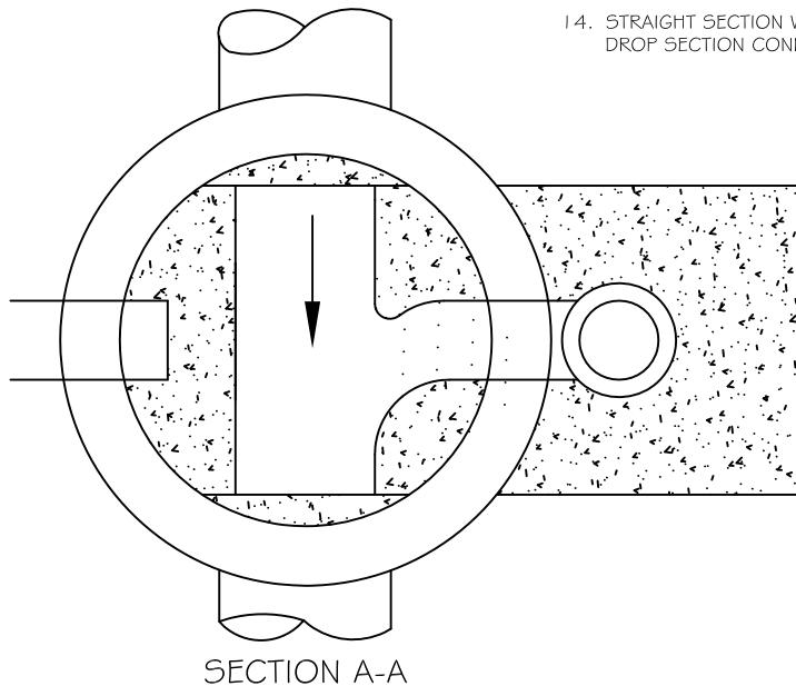
8. CARE MUST BE TAKEN TO FORM A SMOOTH FINISHED TROUGH FROM ENTRANCE PIPES TO EXIT PIPE, AND IN CURVED MANHOLES THE TROUGH MUST BE A SMOOTH CIRCULAR ARC TANGENT TO THE INSIDE WALLS OF THE PIPES AT THEIR ENDS.
